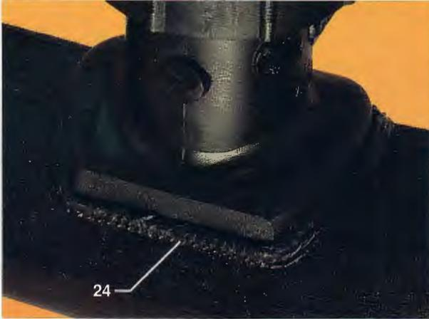
24. Melt Bead Too Small And Insufficient Fusion Pressure
