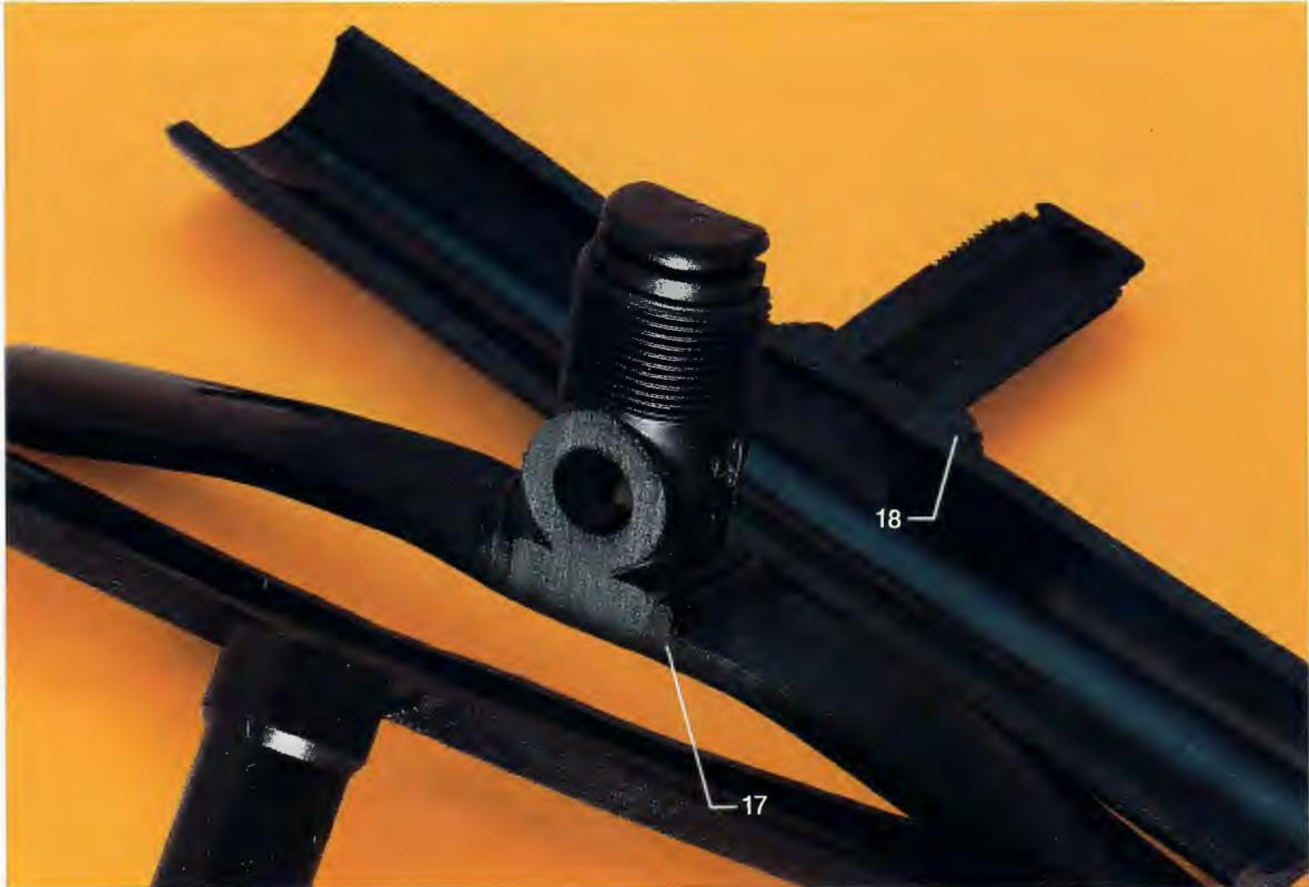
17. Proper Melt, Pressure And Alignment 18. No Gaps Or Voids
