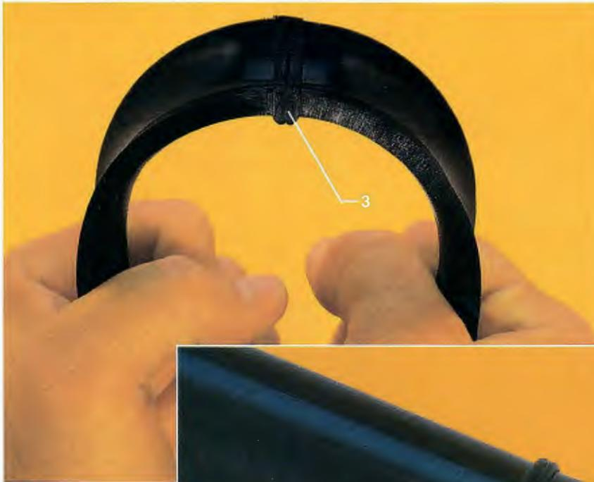
3. Proper Alignment – No Gaps or Voids
