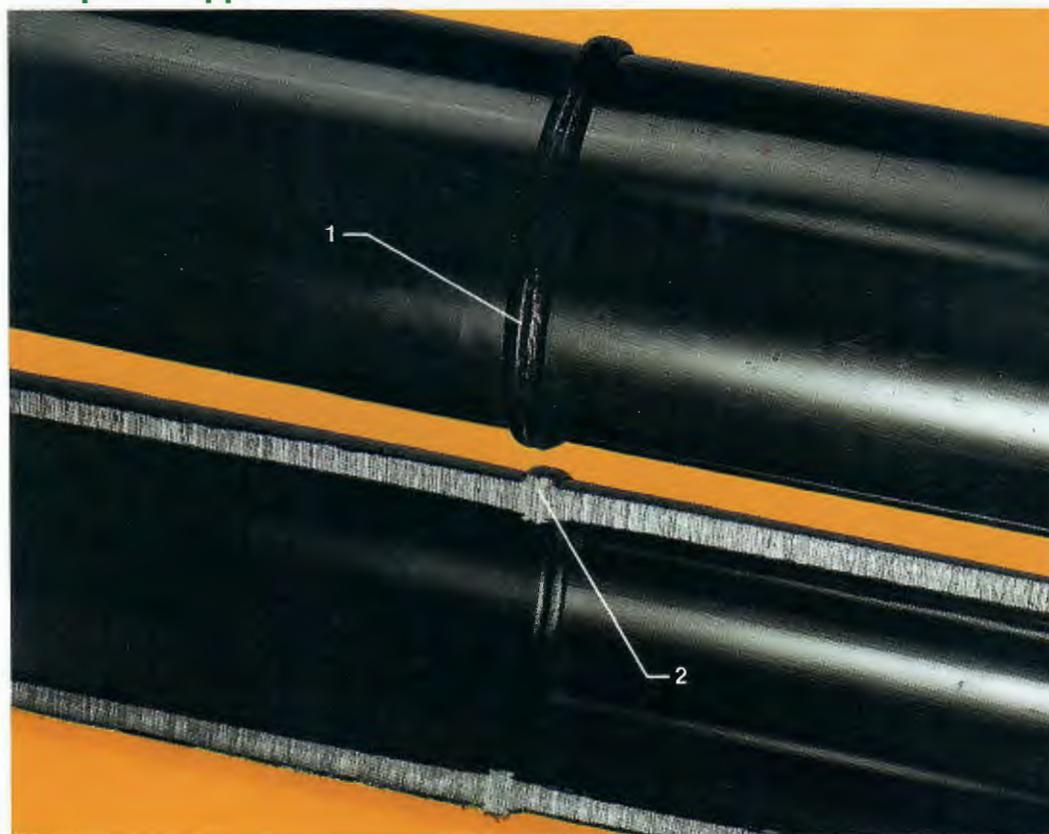
1. Proper Double Roll Back Bead 2. Proper Melt, Pressure And Alignment
