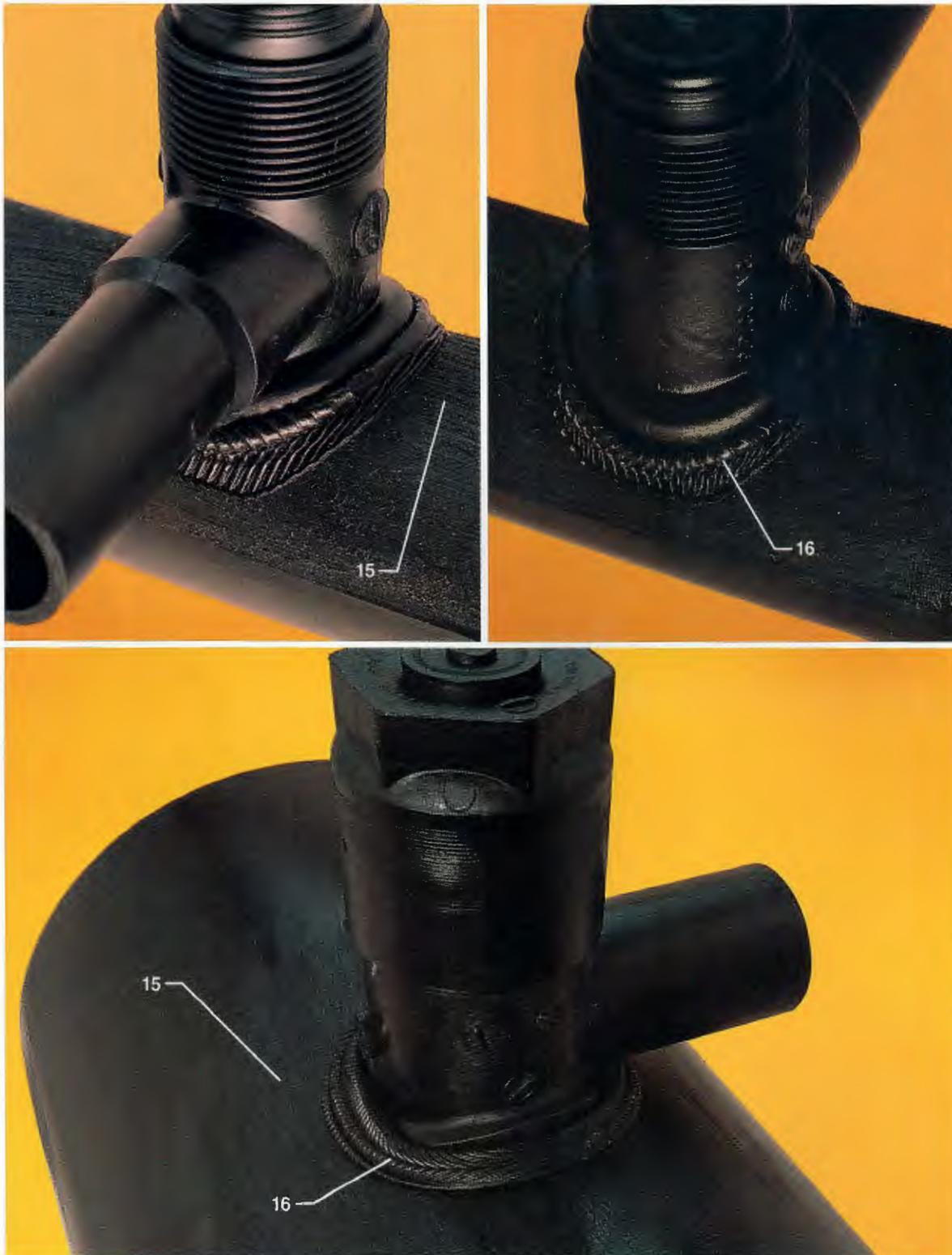
15. Proper Pipe Surface Preparation 16. Proper Melt, Pressure And Alignment
