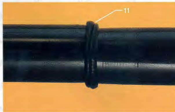
11. Excessive Melt, Improper Alignment And/OR Excessive Pressure
