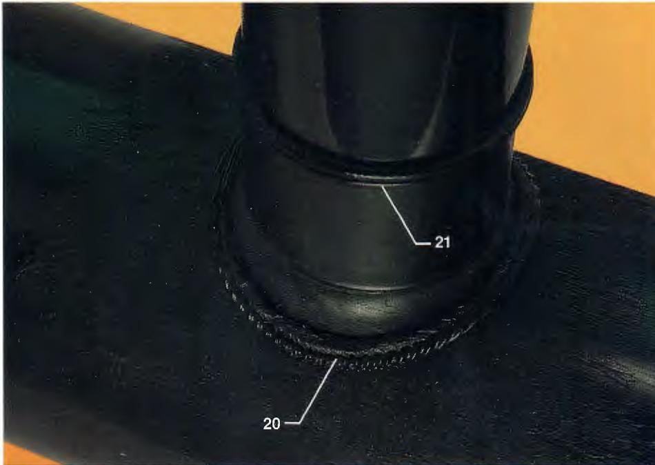
20. Proper Melt, Pressure And Alignment    21. Acceptable Pipe To Fitting Fusion Joint
