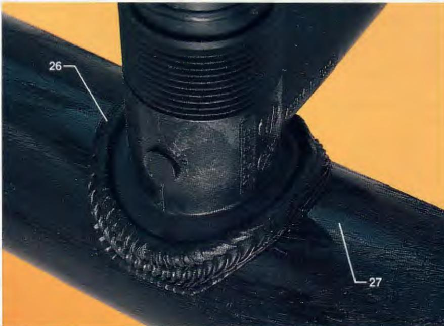
26. Melt Bead Is Above Base Of Fitting 27. Incomplete Pipe Surface Preparation
