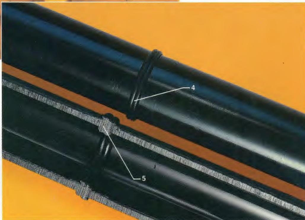
4. Proper Double Roll Back Bead 5. Proper Melt, Pressure And Alignment
