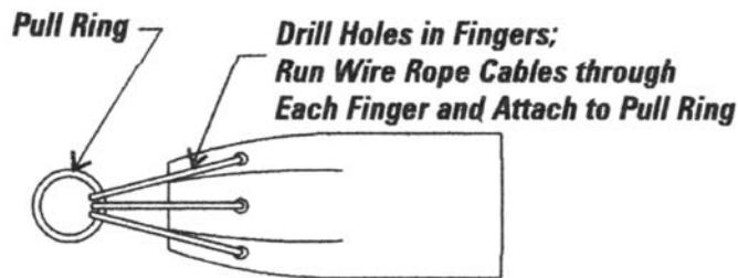
Figure 36 Backhoe Slipliner Push-In Technique
